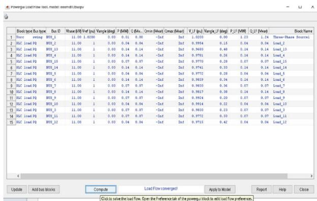
**Figure-9.** IEEE 15 Bus Network Load flow of System without any DG.
