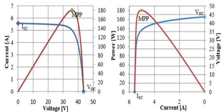
Figure-2. MPPT Curve of a PV Cell
